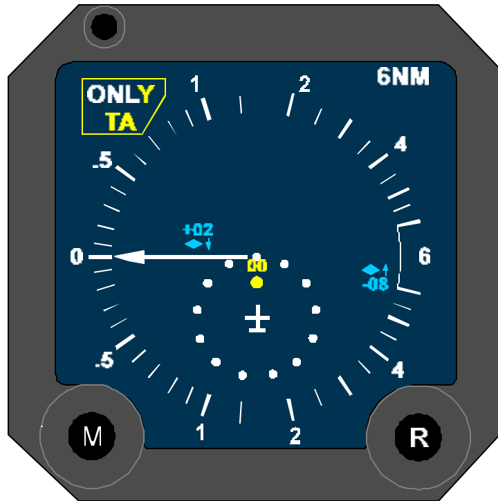
Figure 3B-147. TA ONLY Operational Situation
