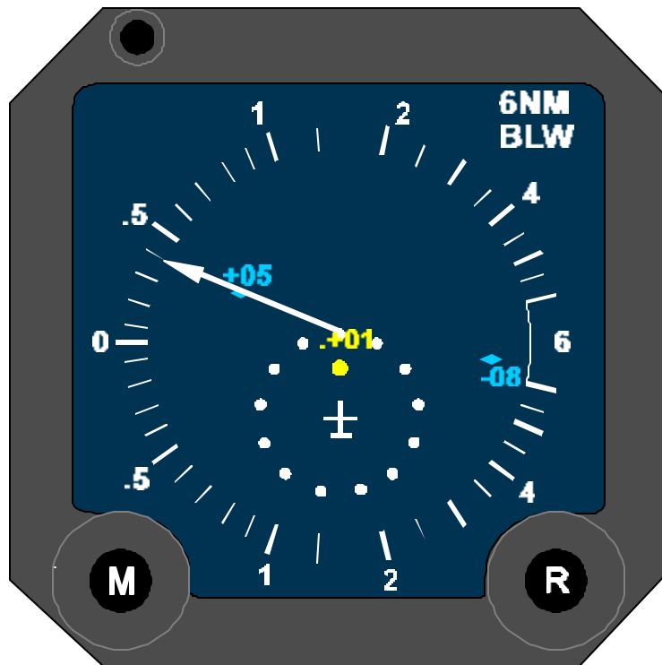
Figure 3B-146. Full Time Traffic Operational Situation
